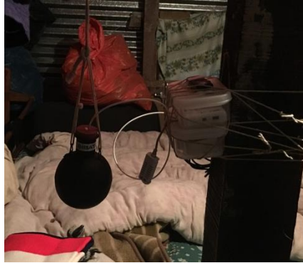
Fig. 2 An examples of installed sensors with data loggers for measuring indoor thermal environment of S1
