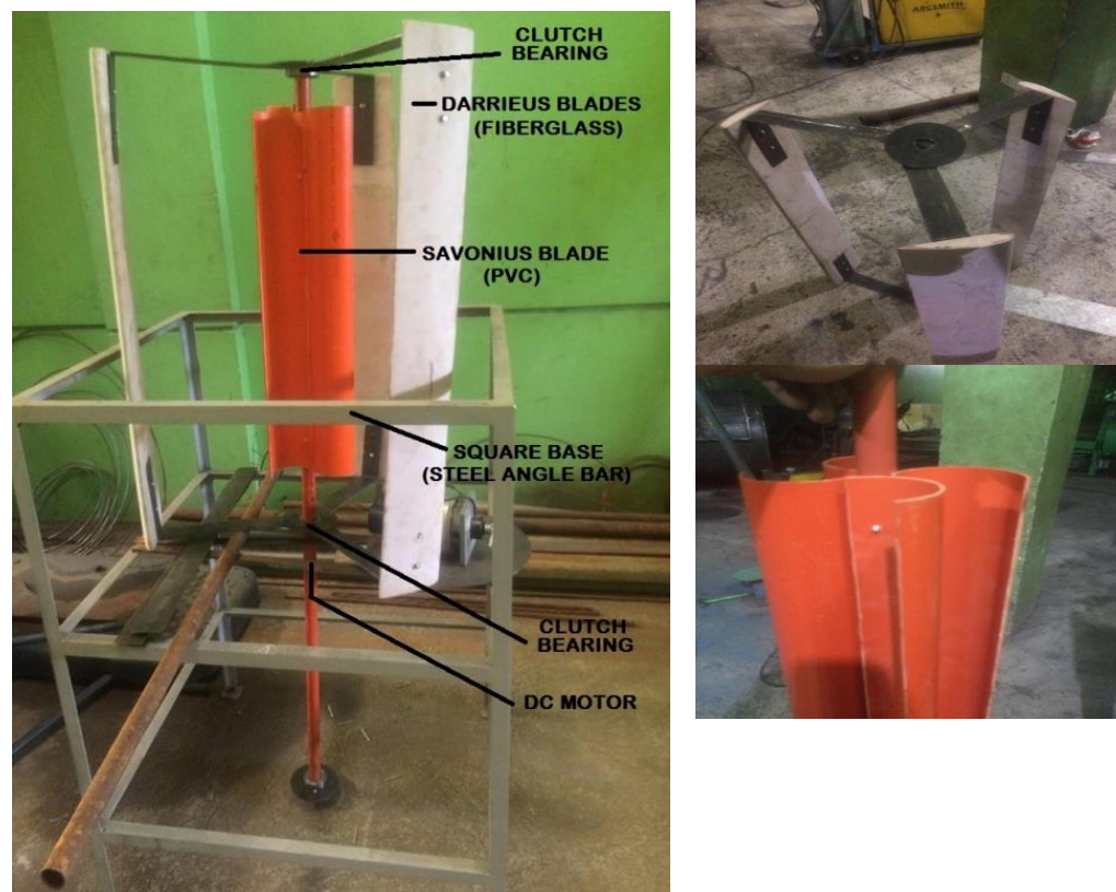
Figure 5. Development of integrated savonius and darrieus small-scale vertical axis wind turbine
