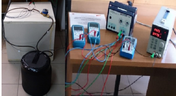
Figure 1. Experimental setup: cooling chamber, water tank and measurement system.
