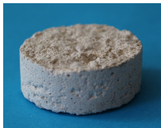
Figure 1. Sample Br after 28 days in 100% humidity
