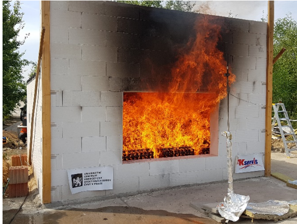
Figure 4. Test room at the 15th minute before the water mist being applied.
