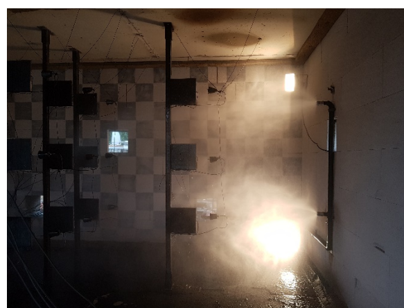
Figure 3. Water mist protection of steel plates.
