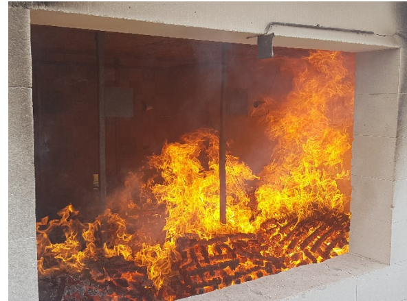
Figure 5. Test room at the 25th minute just before the end of protection.
