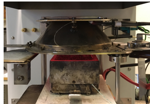
Figure 2. Fire testing of a specimen under the cone heater
