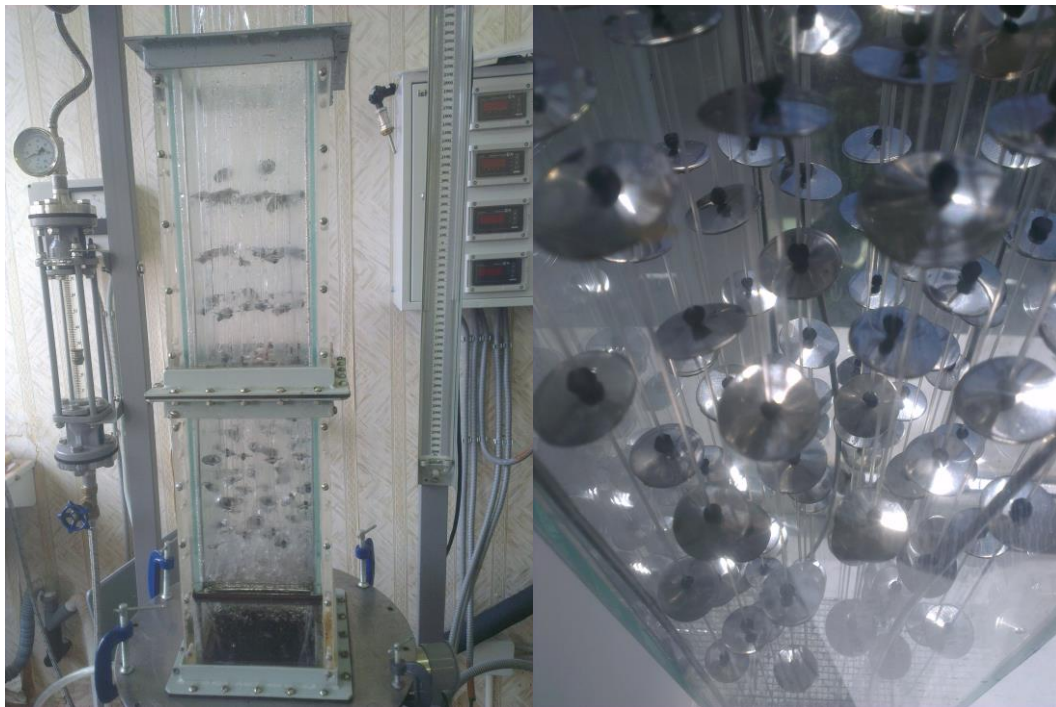
Figure 2. Experimental stand for studying characteristics of packings
