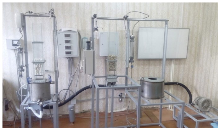
Figure 2. Experimental stand for studying characteristics of packings
