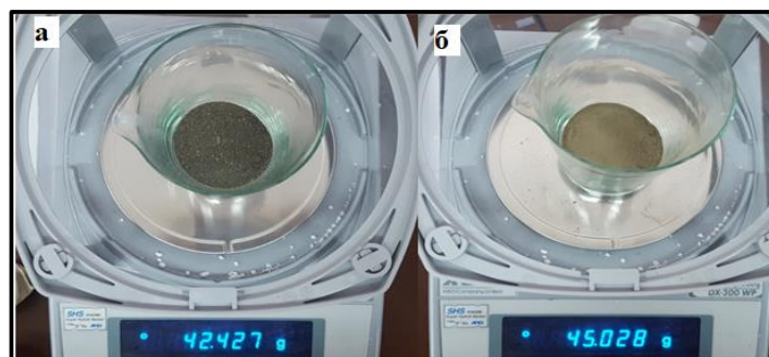
Fig.6 Sample weight without sediment (a) and with sediment (b)
