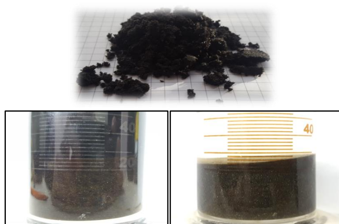
Fig.3 Bitumen saturated, unconsolidated sand of the Ufimian horizon sample. Determination of the sample volume before extraction by immersion in benzene. Determination of the sample volume after extraction by immersion in benzene.
