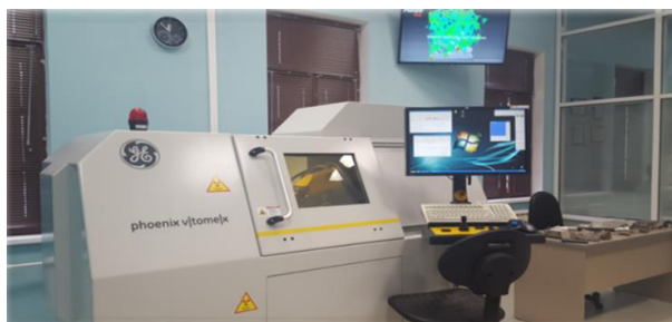
Fig. 1. Micro / nanofocal system for computed tomography Phoenix v|tome|x s240
