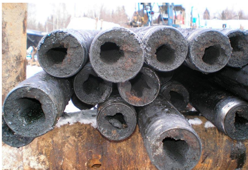
Figure 2. Deposits of asphaltene, resin and paraffin substances.
