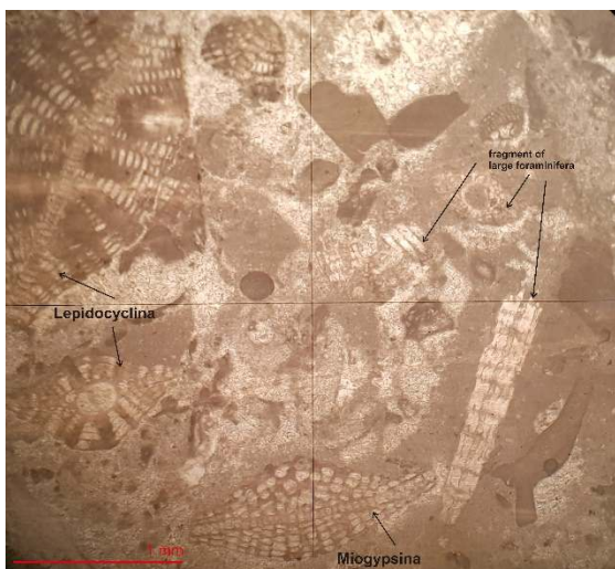
Figure 5. Thin section of Weduar Formation coralline limestone taken from Tamangil area, shows the abundance of large foraminifera.
