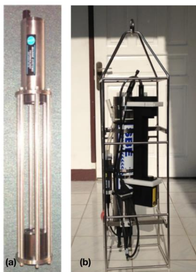
Figure 2. Transmissometer for measurement TSS (a) dan CTD Sensor for measuring conductivity and temperature according to depth (b).
