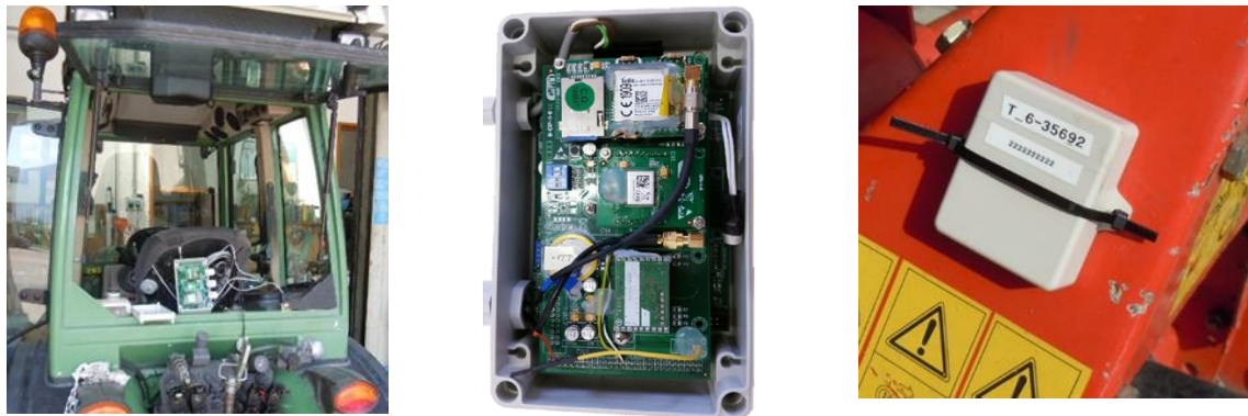
Figure 4. Data acquisition systems details. From the left the first two images show the data logger on the tractor, the third image shows one of the code transmitter on an implement [3].
