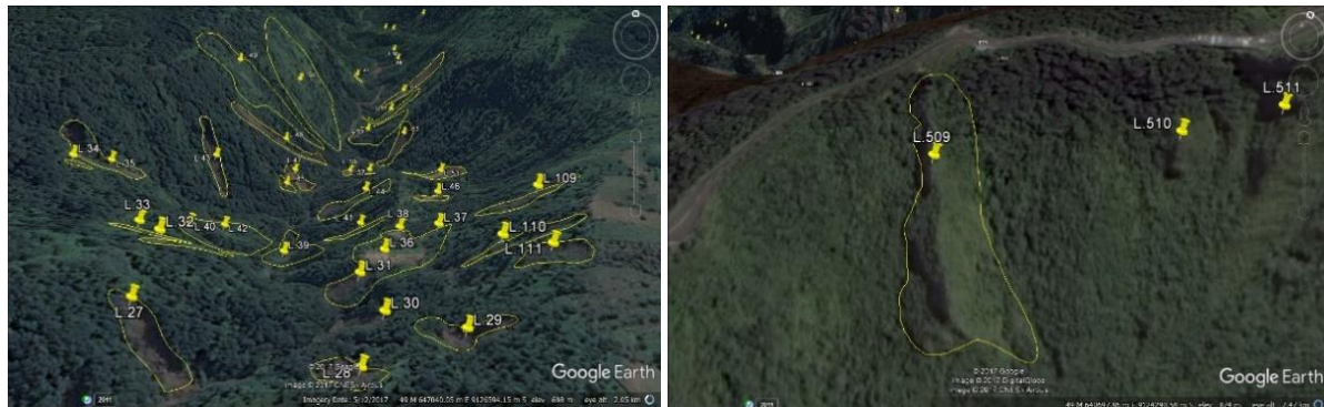
Figure 11. Interpretation Landslide Based on 3D Visualization in Google Earth.
