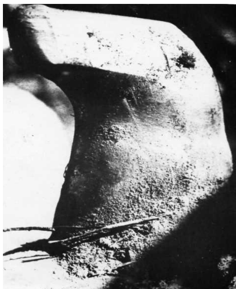
Figure 1. Characteristic wear of cutters.
