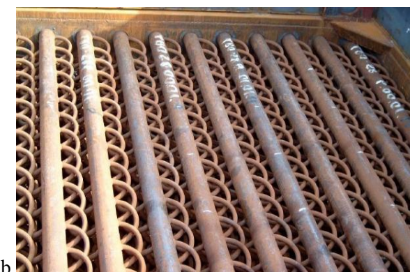
Figure 4. Increased resistance of devices based on SRBT to high temperature loads and deformations (a - straight-tube type, b - SRBT type).
