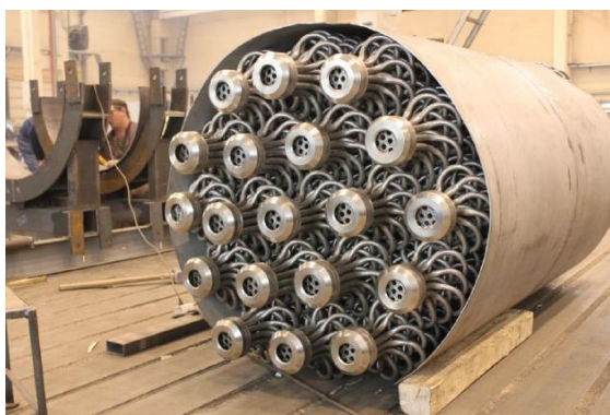
Figure 3. The option of installation of a compact modular design from sections based on SRBT in a cylindrical heat exchanger.
