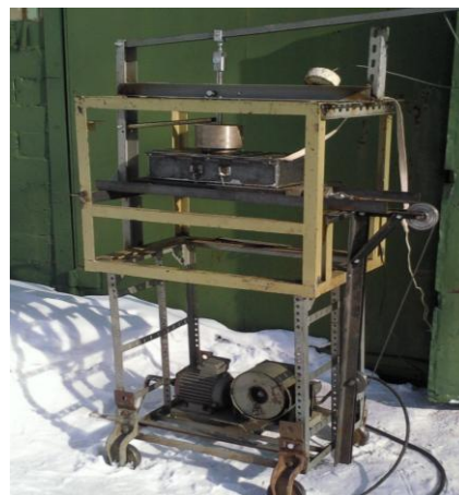
Figure 1. Experimental shear bench for research of thermal effect on soil freezing to metal.
