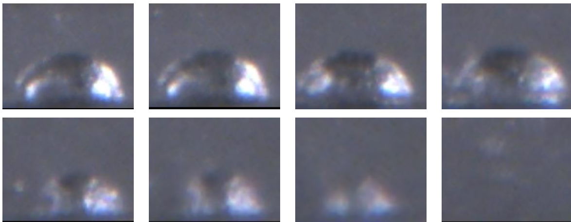
Figure 6. Cavitation bubble collapse process.
