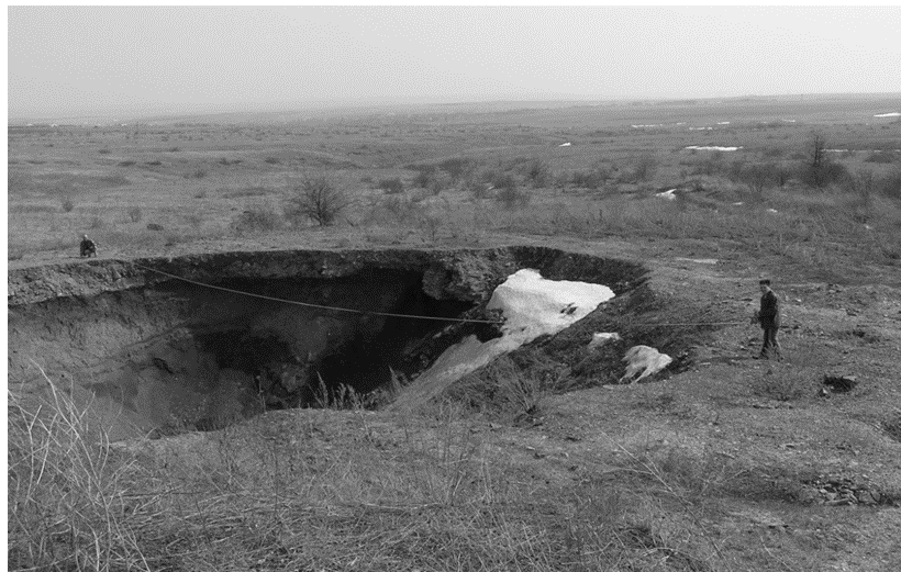
Figure 1. Failure of the earth's surface above the mine workings in the Rostov Region.
