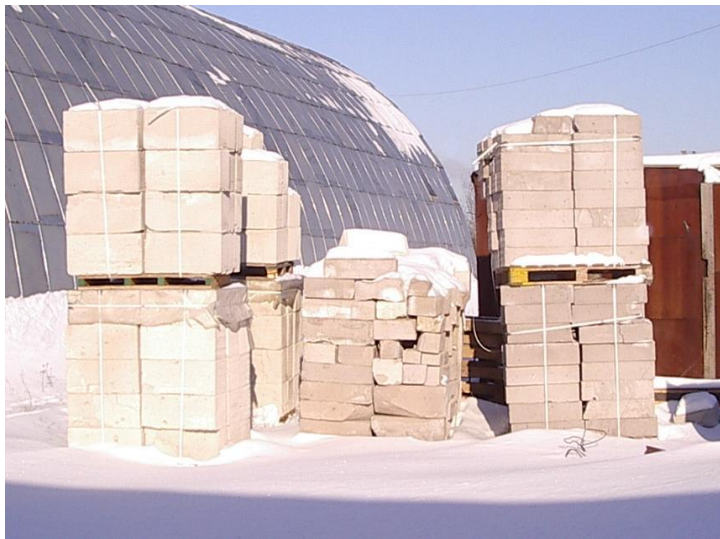
Figure 1. Experimental batches of ash-foam concrete.
