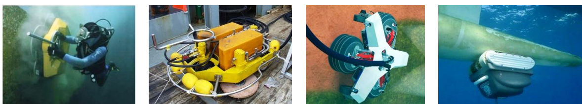
Figure 3. Different types of mechanical cleaning implementation.
