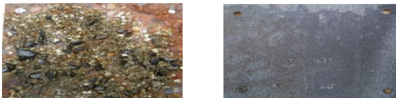
Figure 6. The result of underwater laser cleaning of the test plate from the biofouling (continuous mode, 100 W, velocity scanning 40 mm/s).
