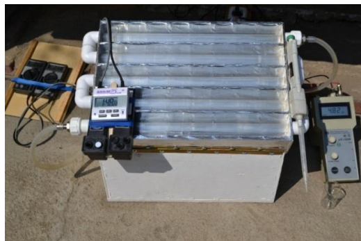
Figure 1. A bench-scale photoreactor unit used in the study
