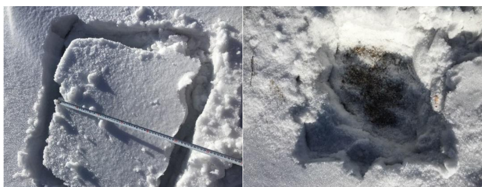
Figure 3. The process of snow sample selection from the open test pit.
