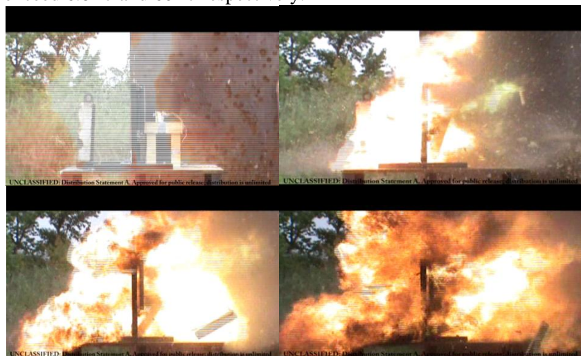
Figure 4. Appearance of fire ball during accidental leakage of HFO-1234yf mixed with lubricant oil in presence of high energy ignition source.
