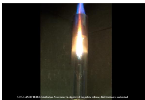
Figure 3. Combustion of “non-combustible” HFO-1233zd(E) in presence of hydrocarbon flame.
