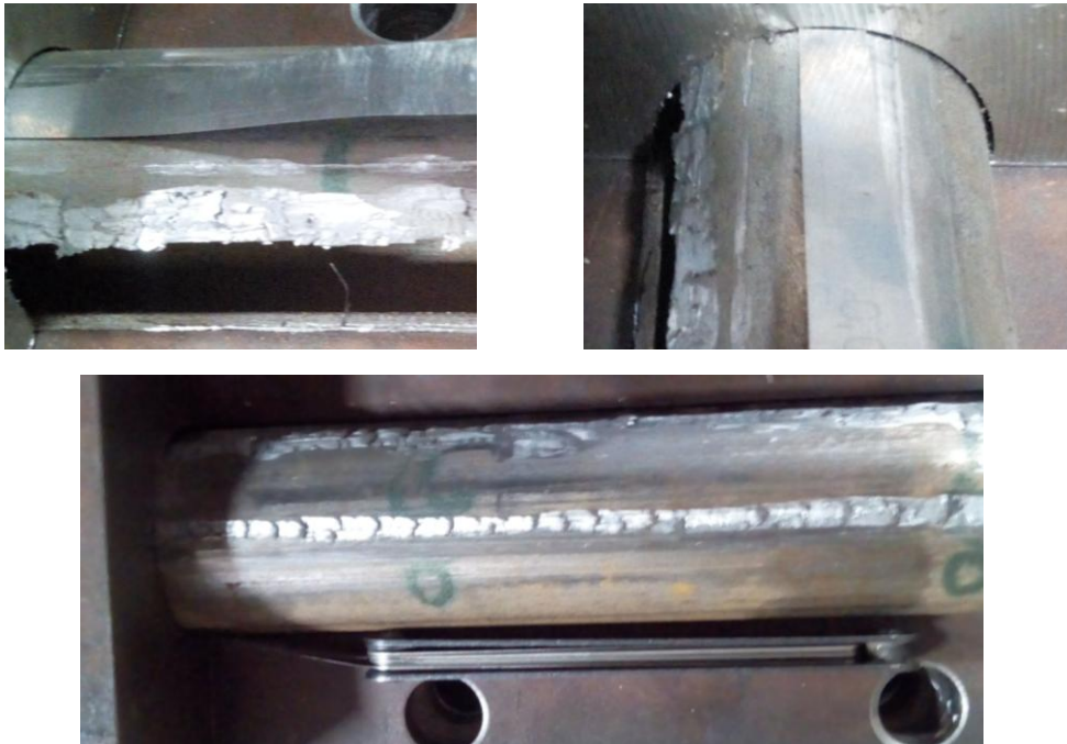
Figure 4. Recording of the state of the anchor rod in the borehole model.
