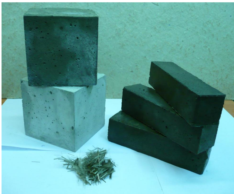
Figure 1. Samples of fiber-reinforced concrete using drilling sludge.
