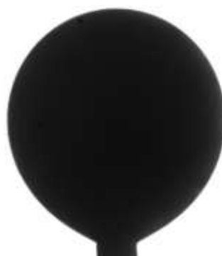
Figure 1. Rising oil drop in IFT cell.
