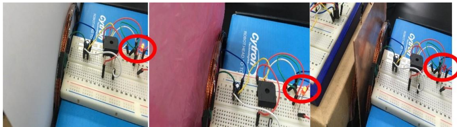
Figure 5. Result of the obstacles (left) paper, (middle) plastic and (right) aluminium between transmitter and receiver coil.
