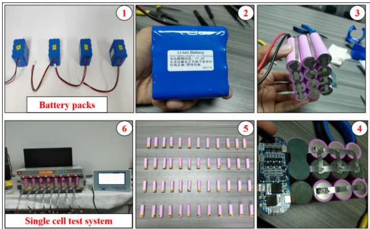
Figure 1. Battery pack dismantling and single cell test process
