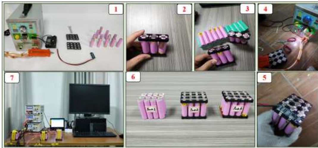
Figure 3. Battery pack forming process and performance test
