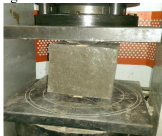
Figure 1 Cube splitting test
