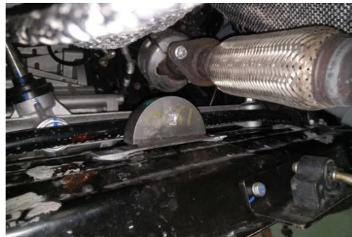
Fig 6.Dynamic vibration absorber installation diagram
