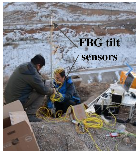
Figure 7. The install of the FBG tilt sensor
