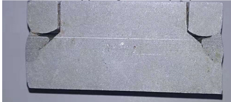
Figure10 Welding arc deflection
