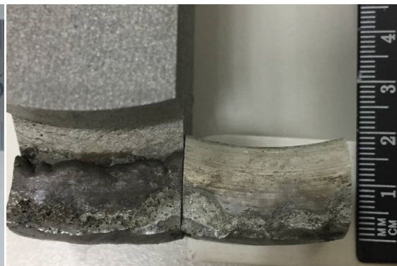
Figure 8 The appearance of welding joint at weld fracture
