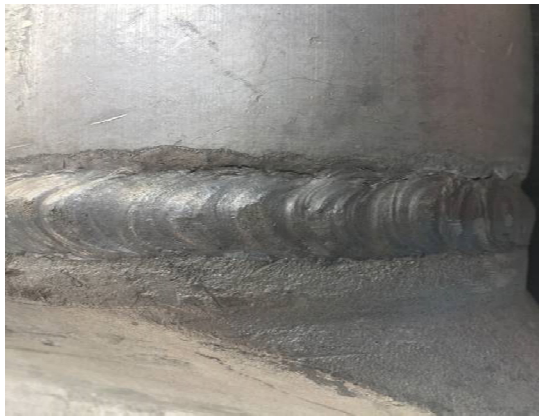
Figure 2 The clamp weld undercut and crack on phase A of #1 transformer
