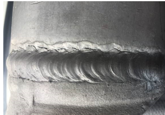
Figure 3 The clamp weld undercut and crack on phase A of #2 transformer
