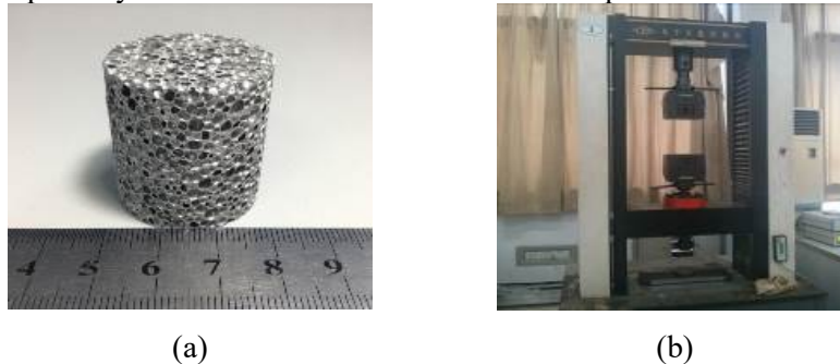
Figure 1. Test specimen and the loading device
