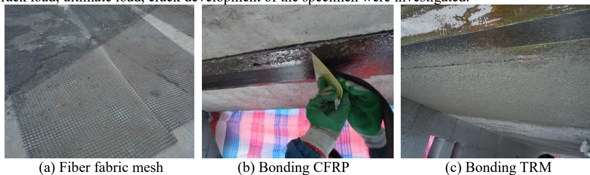
Fig 3. Reinforcement of specimens
