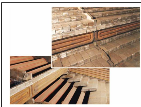
Figure 8. Air cooled grate bars.
