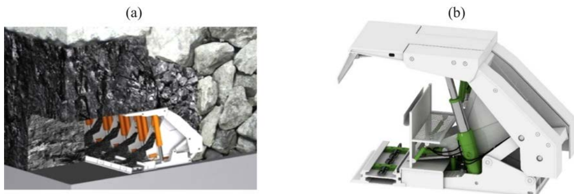
Figure 1. (a) Longwall top coal caving technology in mining thick flat coal seams; (b) general view of powered roof support with controlled discharge of caved coal to armored face conveyor.
