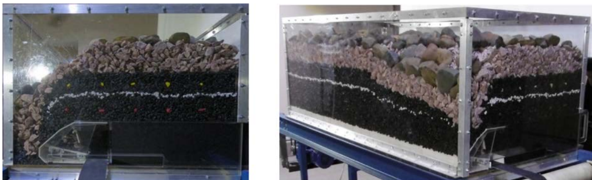
Figure 7. Laboratory testing of discharge flow in different operating modes.
