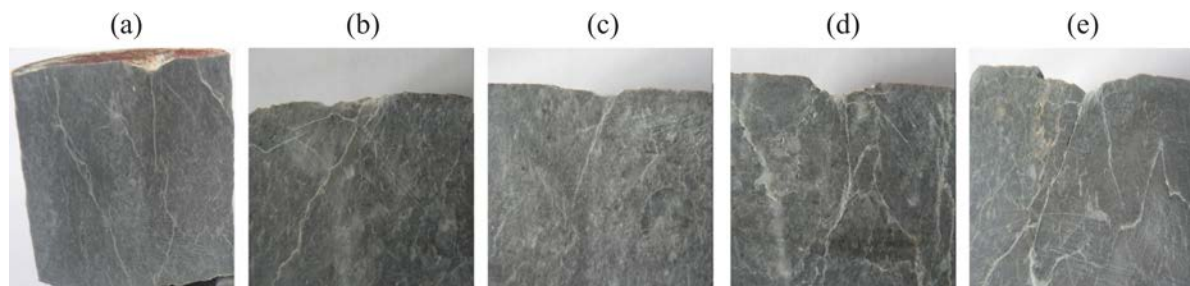
Figure 3. Photographs of polished sections of cores after impacts with an energy, J: (a) 68 (sample blow); (b) 33.6; (c) 68.7; (d) 132.5; (e) 140 (total energy of blows).
