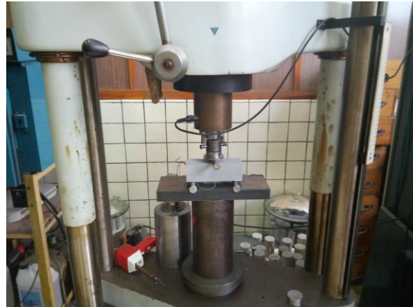
Figure 2. Brenna sandstone beam placed on the pins of the device for performing three-point bending tests.
