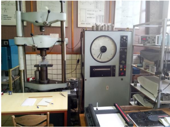
Figure 1. EDZ-40 testing machine with measuring and recording system.
