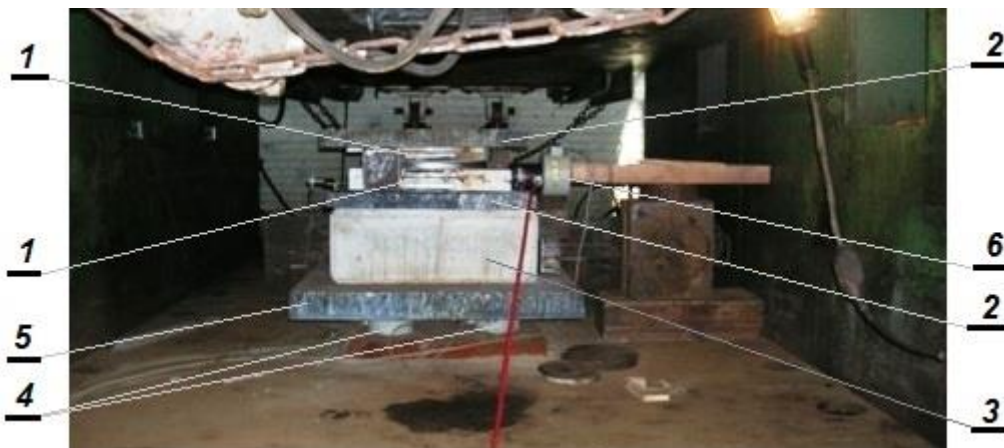
Figure 9. View of arrangement of bearings during determination of friction coefficient on a flat surface 1 – tested bearings; 2, 5 – pressure plates; 3 – transition plate; 4 – transducers; 6 – horizontal cylinder
