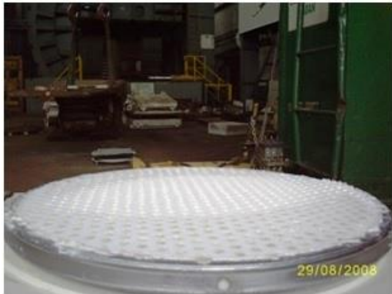
Figure 6. View of the PTFE sheet of lens after bearing capacity test.
