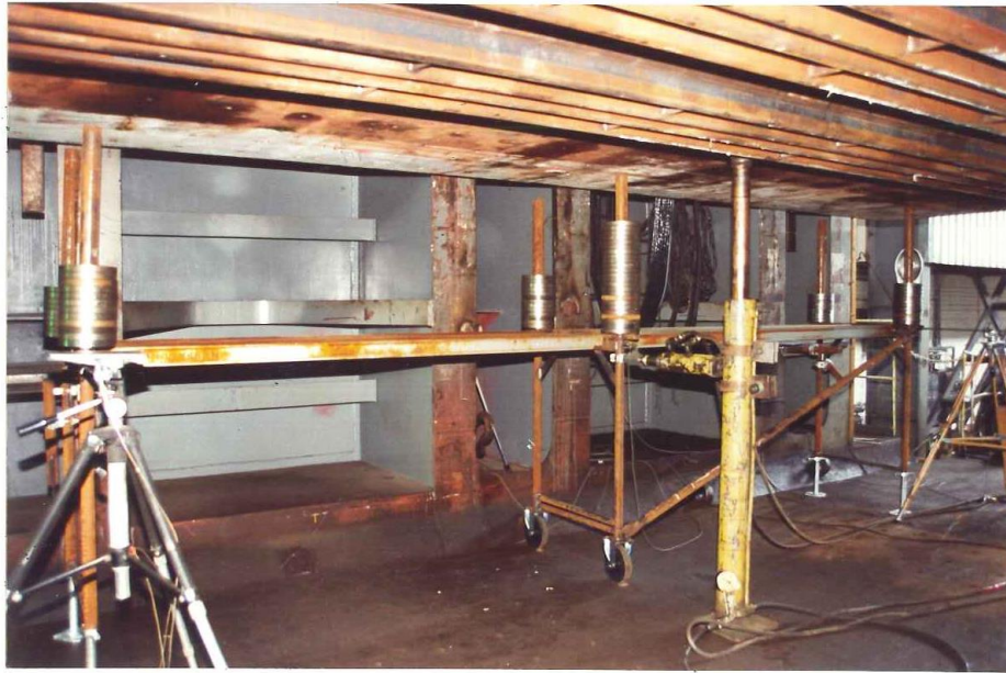
Figure 14. Testing the rigidity of scaffolding with force perpendicular to the platform - general view of the stand.
