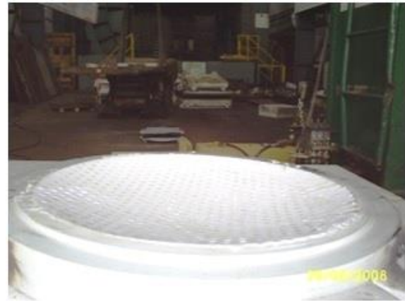
Figure 7. View of the PTFE sheet of the bottom plate after bearing capacity test.
