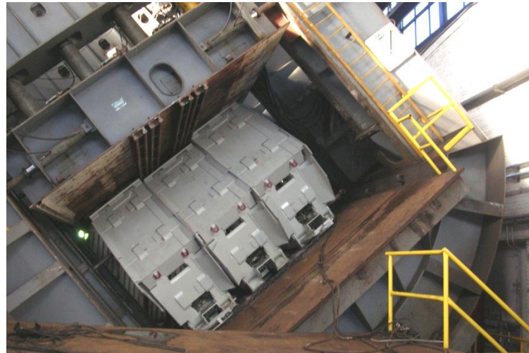
Figure 2. Test stand for kinematic and functionality tests of powered roof support [3].
