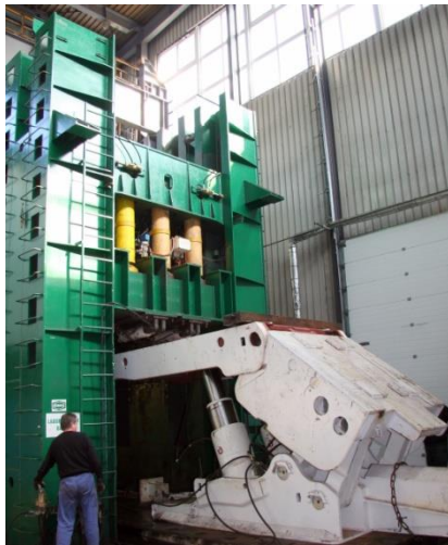
Figure 1. Test stand for strength tests of powered roof support [3].
