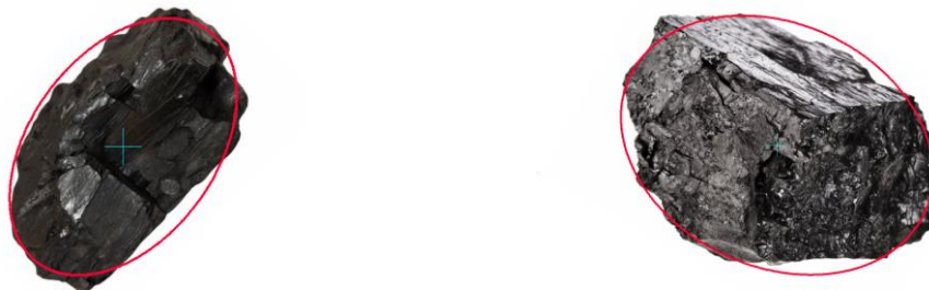
Figure 5. Two examples of elliptical approximation of an elongated and slanted coal particle.
