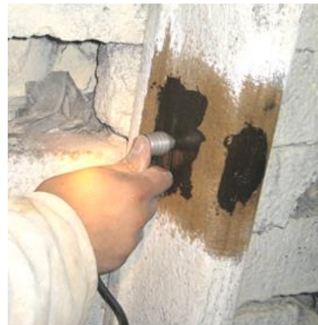
Figure 3. An example of thickness measurement of a section bottom performed "in situ".
