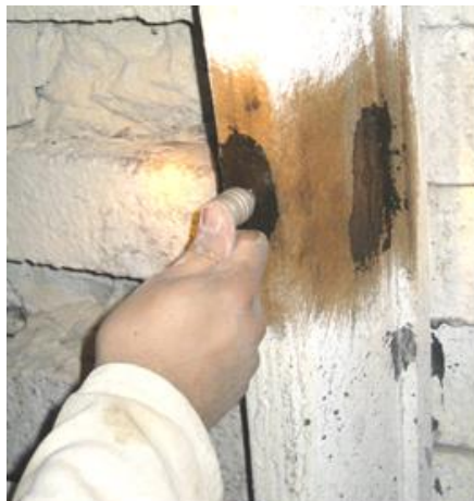
Figure 2. An example of thickness measurement of a section wall performed "in situ".
