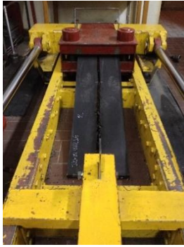
Figure 3. Belt sample after the test.
