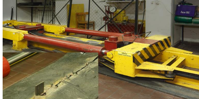
Figure 4. The ZP40 testing machine together with the cutting element.
