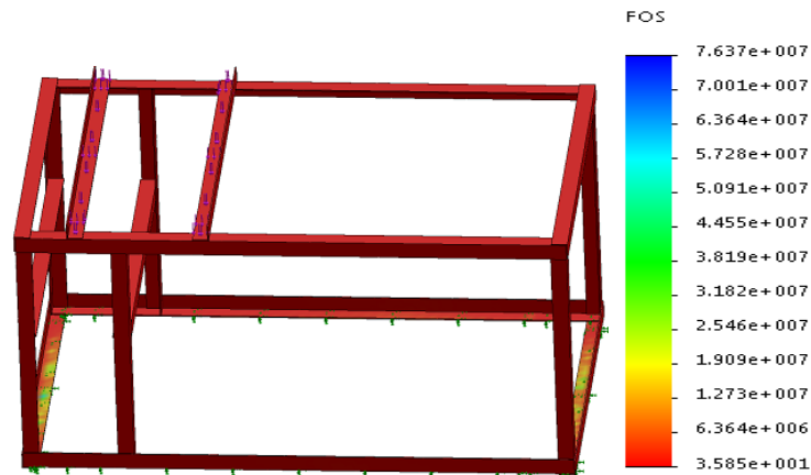
Figure 7. Main frame factor of safety test result
