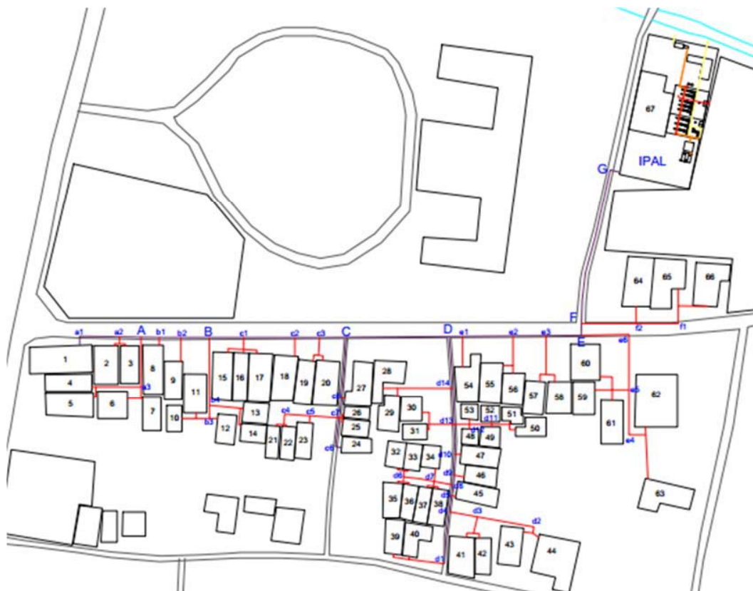
Figure 5. Biogas pipe distribution network from Asri Tofu Factory
