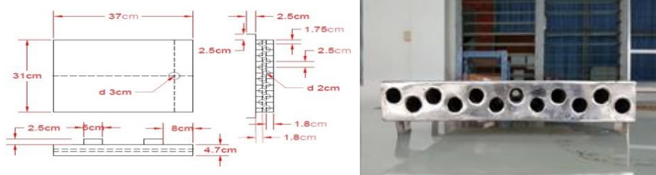
Figure 2. The tube type PCM container.
