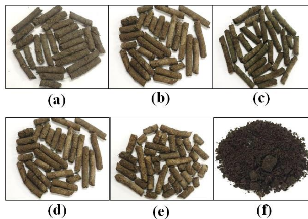
Figure 4. Pelletized filter cake pellets with various initial moisture contents at (a) 40%, (b) 45% (c) 50%, (d) 55%, (e) 60% and (f) filter cake before pelletization with 40% moisture content.
