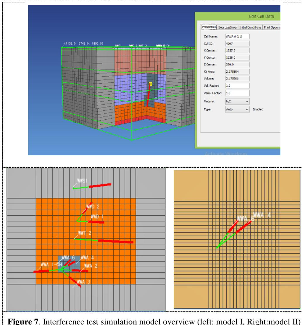
**Figure 7.** Interference test simulation model overview (left: model I, Right: model II)
