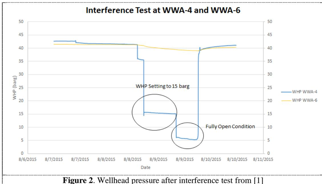
**Figure 2.** Wellhead pressure after interference test from [1]
