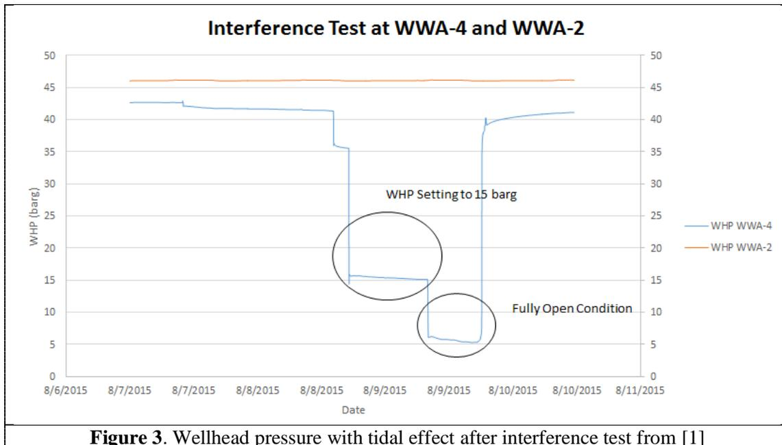
**Figure 3.** Wellhead pressure with tidal effect after interference test from [1]
