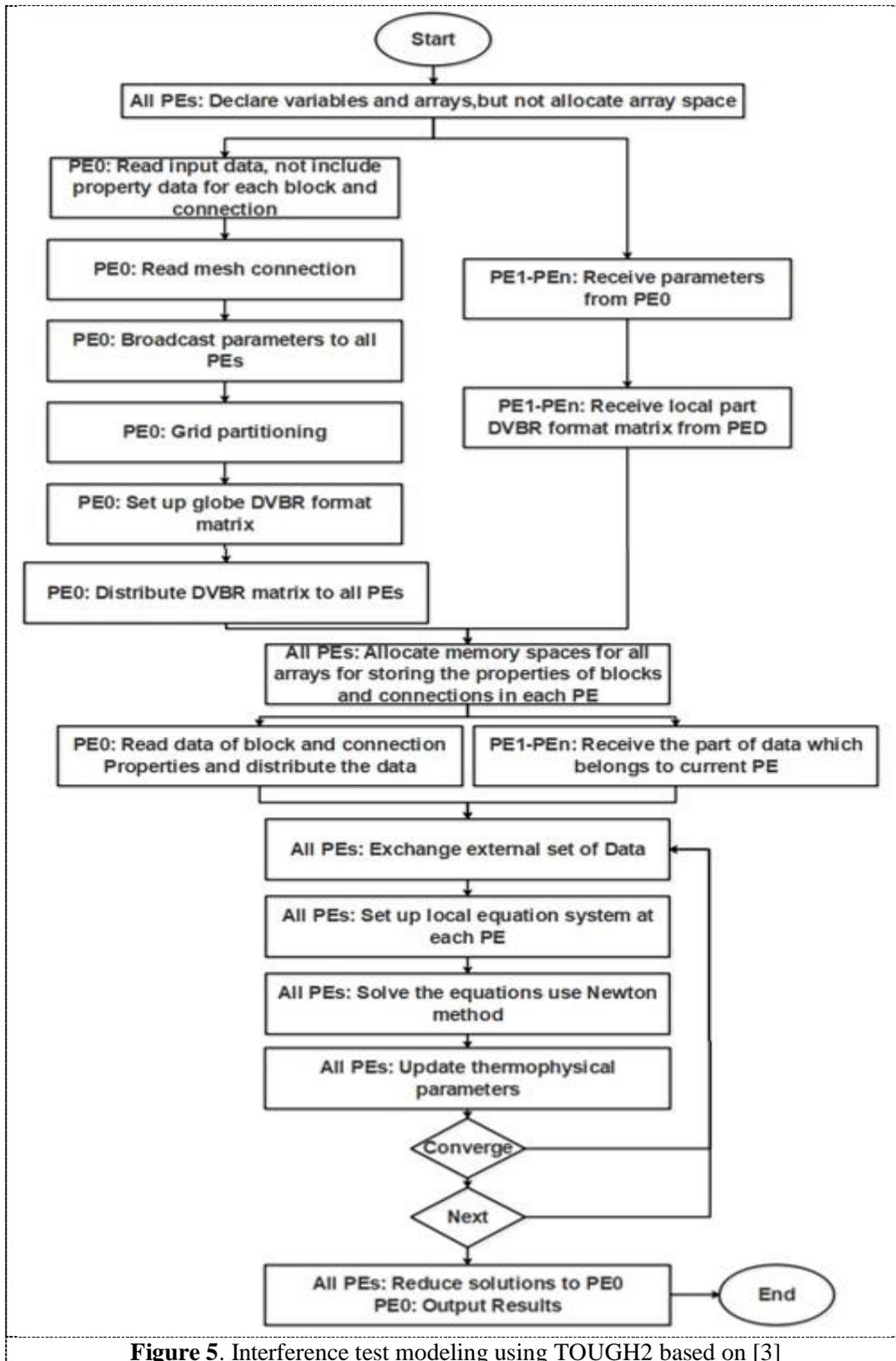
Figure 5. Interference test modeling using TOUGH2 based on [3]
