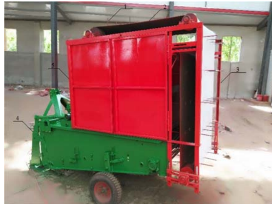
1. The membrane picking device 2. The film feeding device 3. The mounting frame 4. The 4UM-1000 potato harvester 5. The film collecting device
