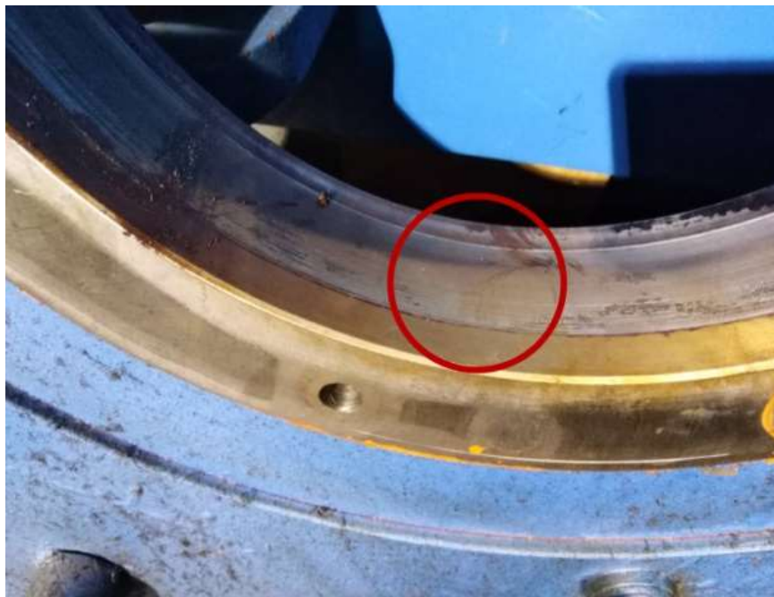
Figure 4. Wear of driving end bearing sleeve
